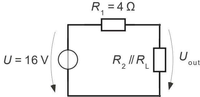
$$R_2 \parallel R_L = \frac{R_2 R_L}{R_2 + R_L}$$
