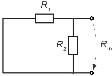
$$R_{in} = R_1 // R_2 = \frac{R_1 R_2}{R_1 + R_2}$$
